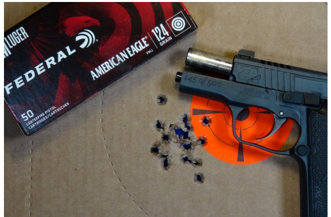
22-rounds of ball ammo inside a 2 ½” group from 7 yards off hand. This consistent accuracy could be due in part to the polygonal rifling in the barrel.
