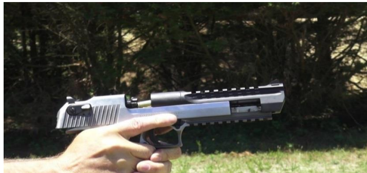
"The author is new to shooting the Desert Eagle, and experienced the well-known 'limp wristing' learning curve that many do. Even with .44 mag as shown here, too soft a grip and stance can induce a feeding failure."
