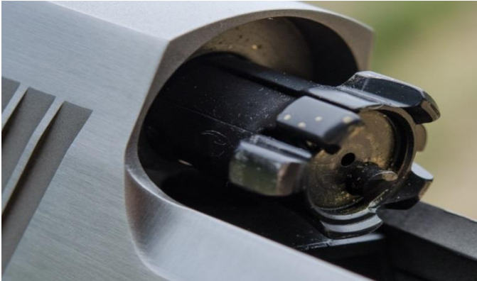
"One of the main reasons the Desert Eagle can handle such high-pressure ammo is the rotating bolt design."
